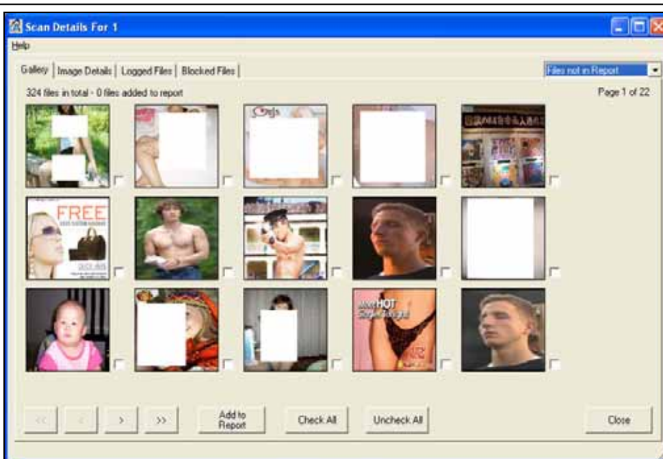
The porn detecting results of a skin-tone based porn filter: PixAlert ( http://www.pixalert.com/ ). Many innocent images were classified with high scores of porn.
